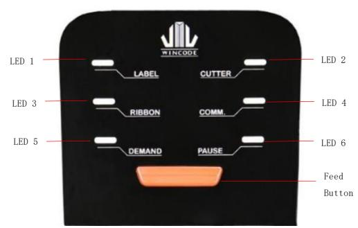
LP423N/LP433N model is equipped six functional LED indicators (blue color) and a feed button (white and red LED color), user can understand the current printer status easily according to the LED display status. The description of each LED display status is listed as follows.
